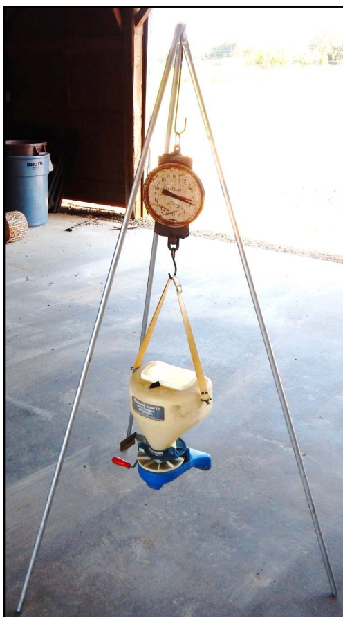
Figure 7. A milk scale, or a similar scale, can be used to weigh the spreader.
