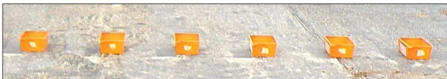
Figure 2. Layout of catch bins, two feet apart, on center.
