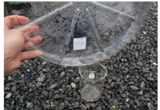
Pour leachate into a container that is deep enough to hold the test probe.
